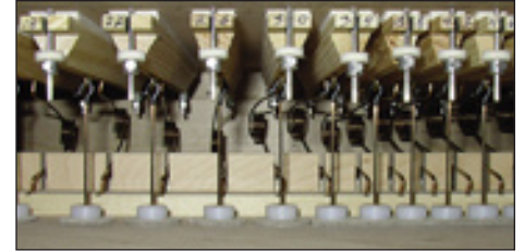
Each time a key is pressed one of these valves in the windchest opens.
